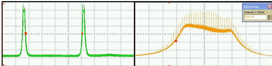
4μs Gain-switched pulses of 11.1kHz (without filter) Gain-switched pulse with filter with 200ps overlapping pulses
