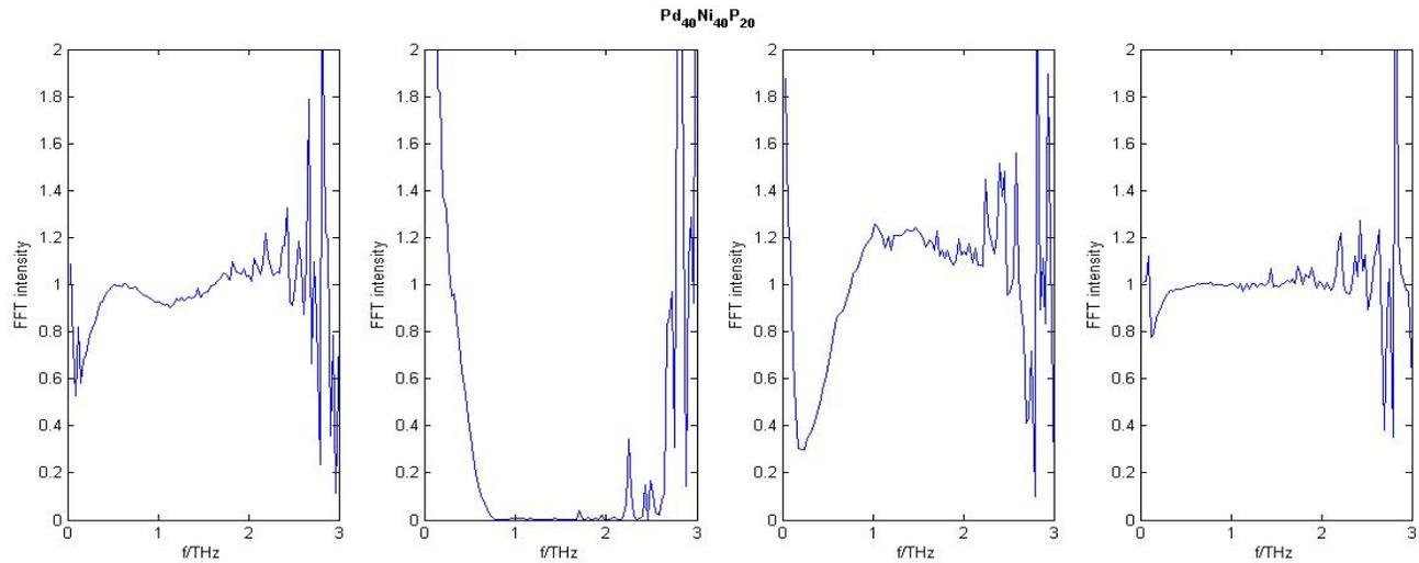
FIG. 3. Transmission factor for Pd<sub>40</sub>Ni<sub>40</sub>P<sub>20</sub>. **Left:** Beam hitting the sample in one edge. Note an absorption peak around 0.35 THz. **Left center:** Beam hitting the sample, showing almost full absorption. **Right center:** Beam hitting the sample in the opposite edge, showing a much more prominent absorption peak around 0.35 THz. **Right:** Beam outside the sample.
