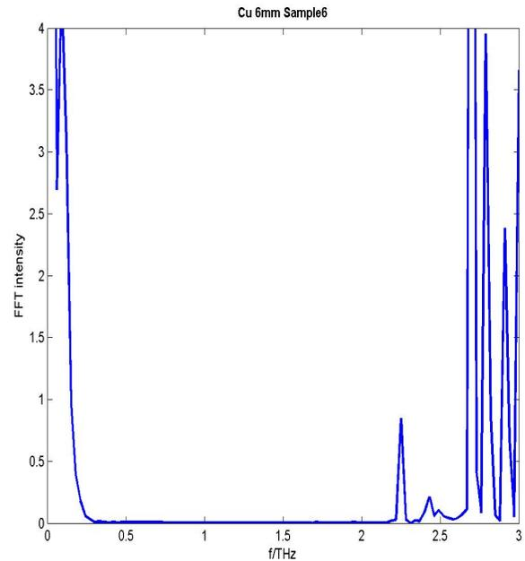
FIG. 5. Transmission factor for pure Cu 6mm wide. Unlike other ribbons, which wide was about 1mm, the transmittance is almost zero. This shows the important role the diffraction pattern plays in our measurements.
