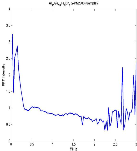
FIG. 4. Transmission factor for  $\text{Al}_{85}\text{Ge}_{10}\text{Fe}_3\text{Cr}_2$  metallic glass sample, dated on 21/1/2003. The sample does not show an absorption peak at low frequencies.
