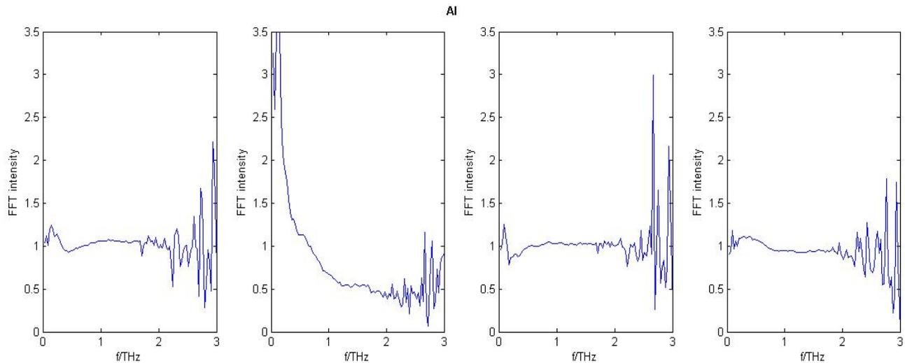
FIG. 2. Transmission factor for pure Al. **Left:** Beam outside the sample. Noise becomes important above 2 THz. **Left center:** Beam hitting the sample, showing almost null transmission. **Right center:** Beam hitting partially the sample, showing no absorption peaks. **Right:** Beam outside the sample.
