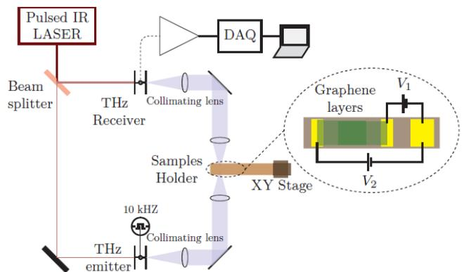
FIG. 1. Schematic view of the THz time-domain experimental setup employed to characterize the samples illustrating the disposition of the samples and voltage sources.
