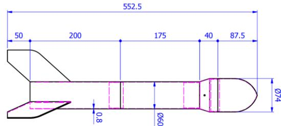
FIG. 1. Design of the rocket made with Autodesk Inventor.
