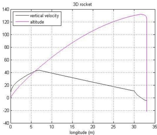
FIG. 4: 3D rocket trajectory in meters (purple) and sinking rate in meters per second (black).
