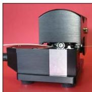
**Tapping in** A simple piece of equipment can be used to listen in on optical-fibre communications.
